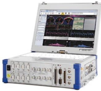
16 channels MDAQ (8 DSUB, 8 BNC)
