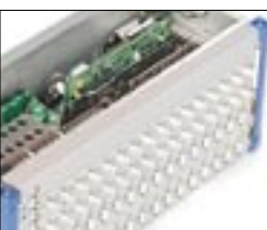
Typical application: 64 ch. DEWE-501 with built-in DEWE-ORION A/D cards
