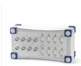
DEWE-31-16: 16 channel signal connection with MDAQ signal conditioning
