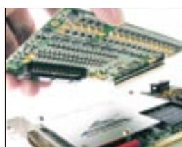
DEWE-ORION-3216-10x 32 channel PCI A/D board (1616 with additional inputs)
