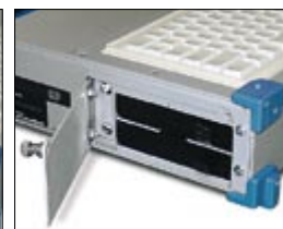
Hot swappable battery exchange
