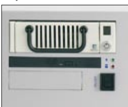
BAY-5.25 Prepared for a removeable HDD
