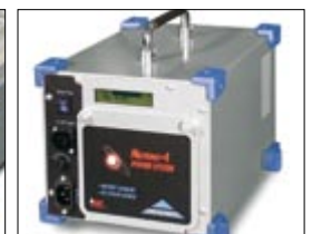
Neutrino-4: charge batteries independent from DEWE-3108
