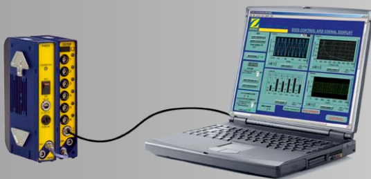
Miniature system Single module system with direct link to the PC via USB 2.0
